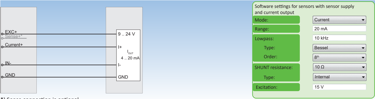
Fig. 106: Sensors with sensor supply and current output
